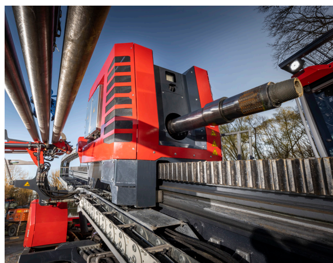
Figure 2. The system of HDD80-E is constructed as electrical in its entirety.
