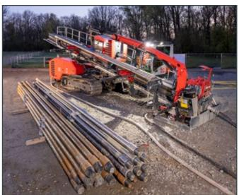
Figure 1: HDD80-E –STREICHER's fully-electric driven HDD rig
