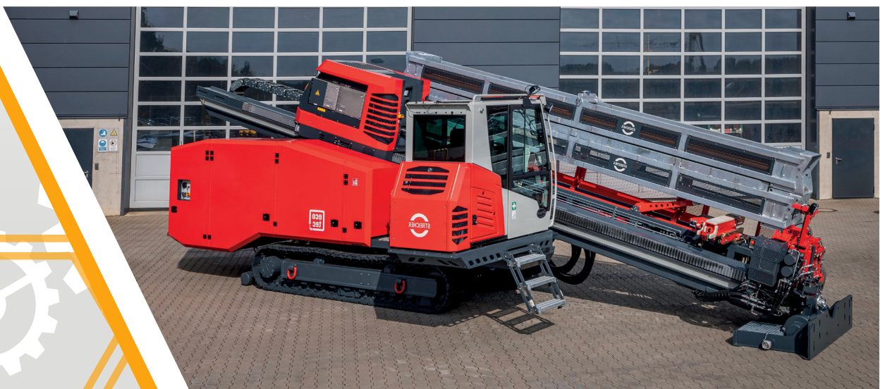
Figure 1. Fully electric driven horizontal drilling rig HDD45-E.
