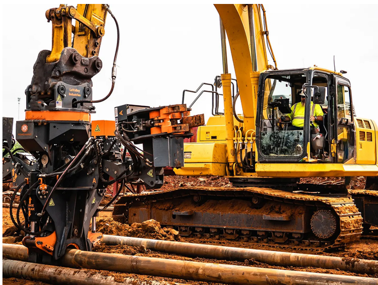
LaValley Industries: LaValley Industries' TONGHAND® mechanised torque management system controlling torque, alignment, and load position during HDD exit-side operations, with the operator positioned in the cab and separated from the immediate risk zone during high-energy transitions.
